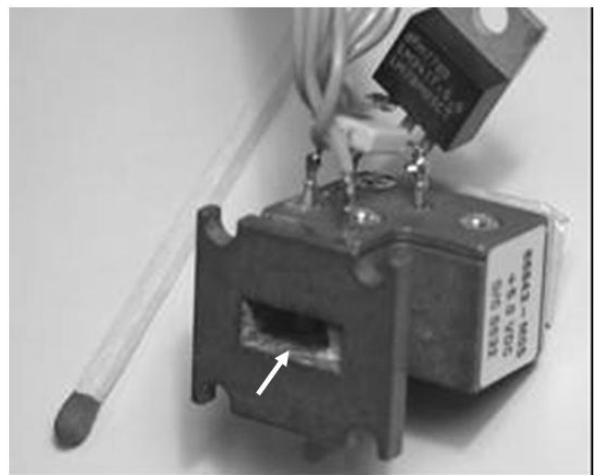
Figure 11. Stray current corrosion of a micro wave module for 24 GHz used in a control equipment.
